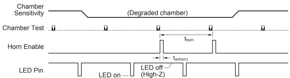
Chirps occur after 2 consecutive failed tests, and are offset from LED flashes and from chirps that indicate failure of low-battery tests
